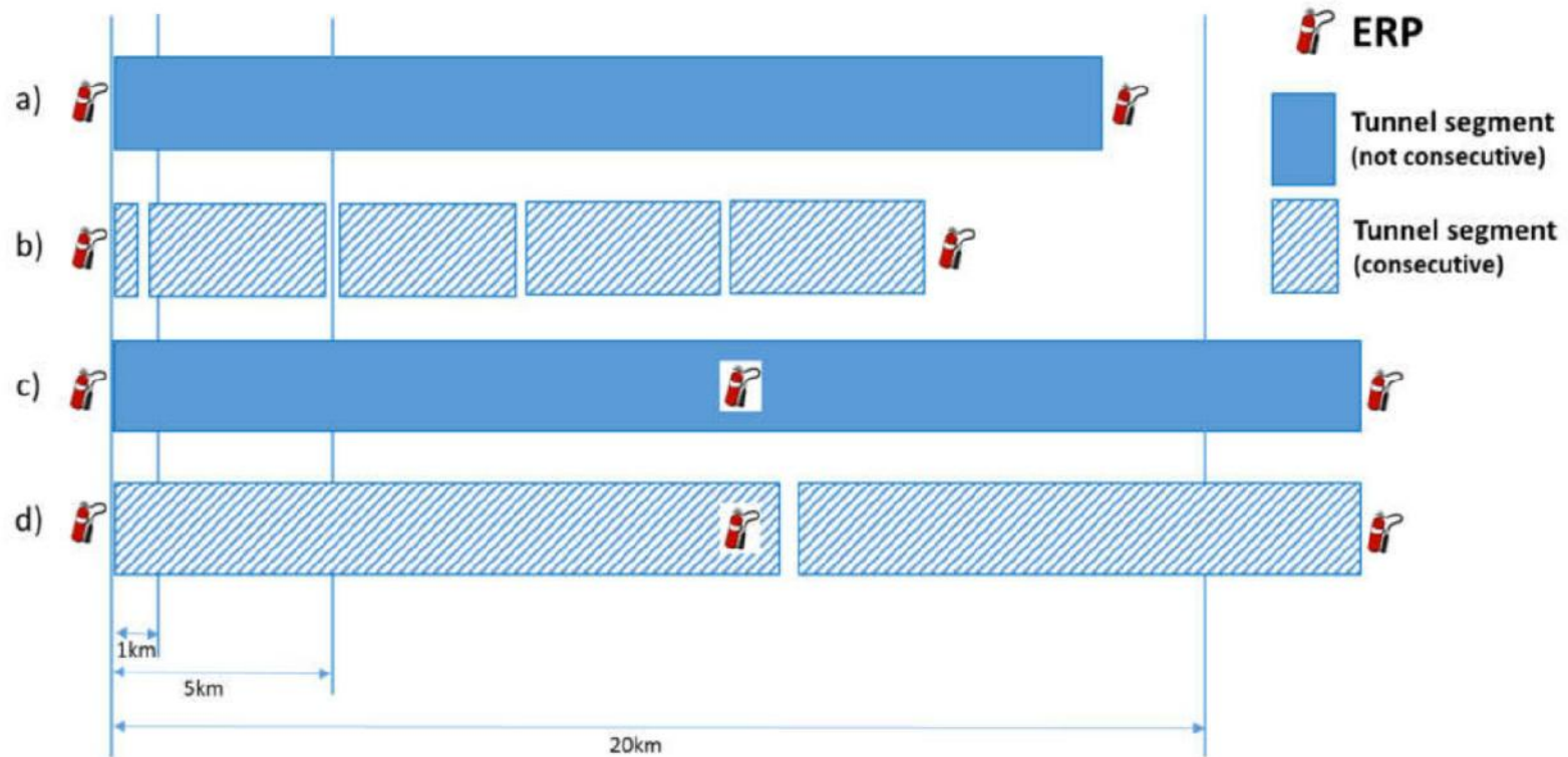
Figure 4 Examples of configurations of evacuation and rescue points and tunnels for lines accepting only category B trains
